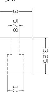
TB-10 is molded from a nylon & polyester fibre reinforced rubber of 80 (+ or -) 5 durometer, and has an average impact resistance of 95% under ASTM 1170.
