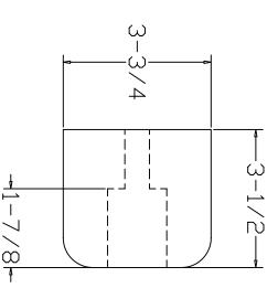
average impact resistance of 95% under ASTM 1170. polyester fibre reinforced rubber of  $80 \ (+ \ or \ -) \ 5 \ durometer, and has an$ TB-20 is molded from a nylon &
