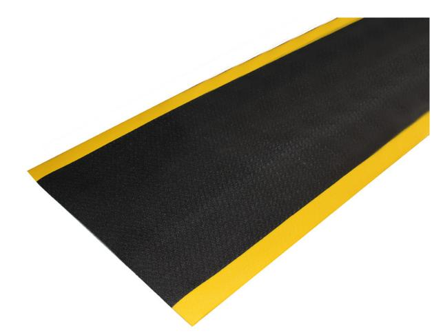
Polyurethane top coated mat provides improved resistance to abrasion and chemical resistance. Non-directional, pebble surface is easier to clean than non-coated products. Cushioned comfort to minimize leg fatigue. Resistant to many common fluids and chemicals. 100% chemically blown, polyvinyl chloride foam with a surface coating of heavy duty polyurethane provides durable, extended service and easy maintenance.
